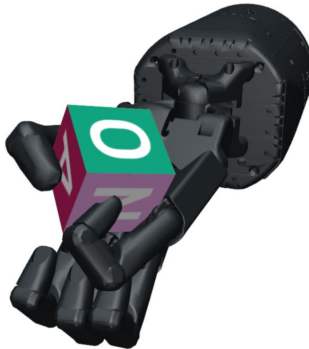
Figure 1: A Simulated Anthropomorphic Robotic Hand Performing In-Hand Object Manipulation
