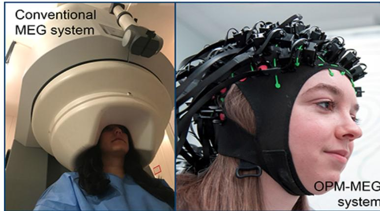
Figure 33. Comparison between conventional MEG and OPM-MEG system (source: <https://www.birmingham.ac.uk/university/colleges/eps/news/2021/an-interview-with-cerca-developers-of-the-world's-most-accurate-brain-scanner.aspx>)
