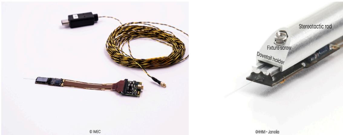
Figure 14. Neuropixel probe integrated silicon CMOS digital neural probe with on-chip circuitry for signal conditioning and digitization (source: <https://www.neuropixels.org/probe>)
