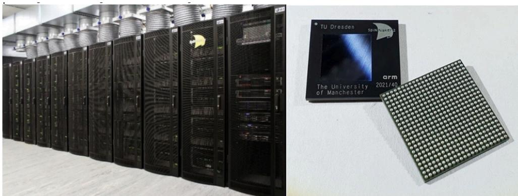
Figure 91. SpiNNaker-2 system (left) and chip (right) (source: EBRAINS)
