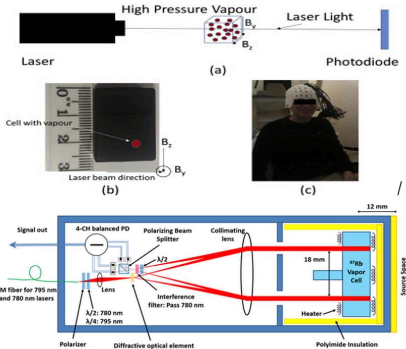
Figure 31. The OPM sensor's schematic. depicts the scheme of an OPM sensor. PBS: polarising beam splitter; PM: polarisation maintaining, PD: photodiode,  $\lambda/2$ : half wave plate,  $\lambda/4$ : quarter wave plate. (Source: <https://doi.org/10.1371/journal.pone.0227684.g002>)
