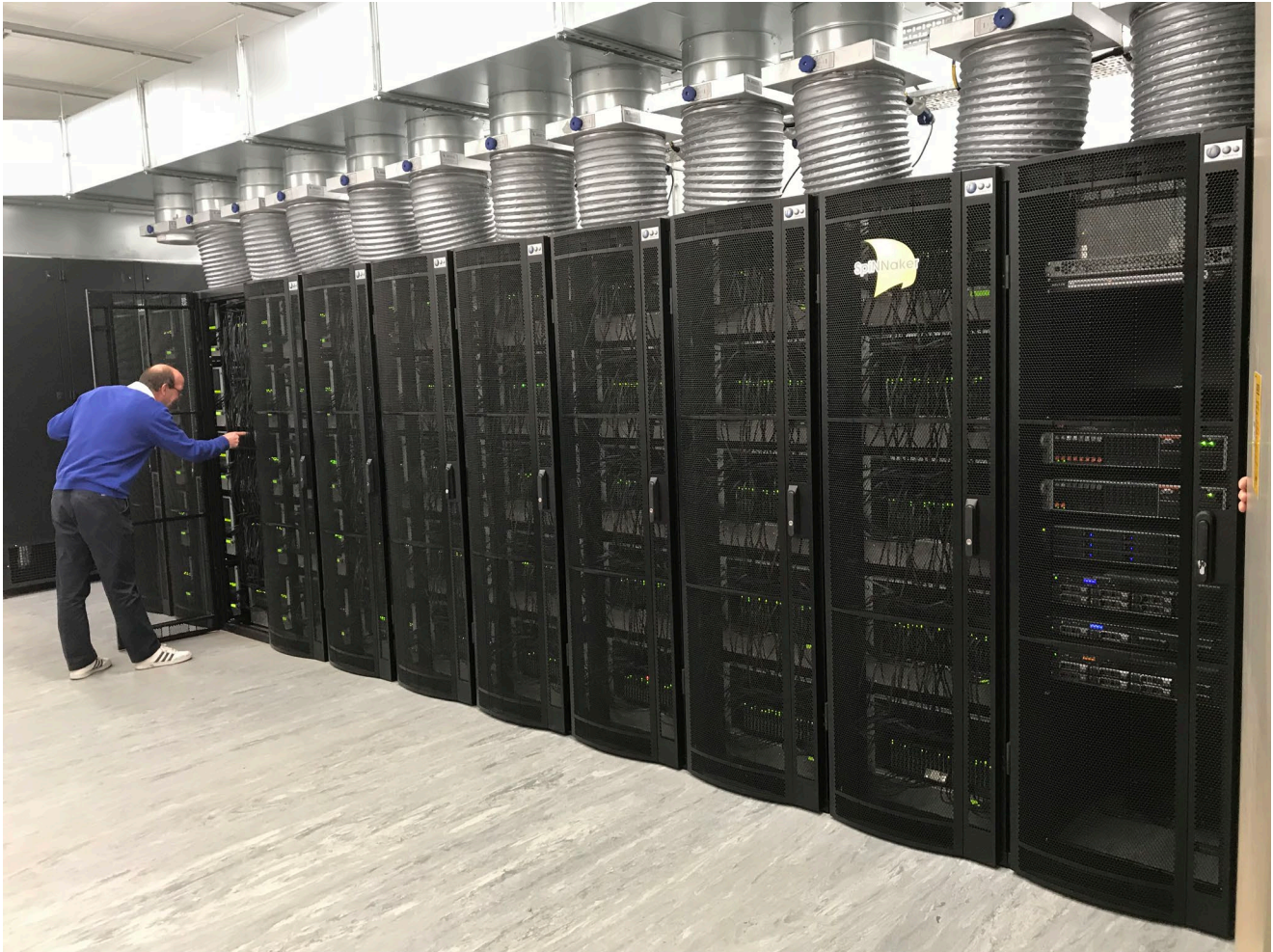
Figure 7: The million-core SpiNNaker machine at UMAN that supports the EBRAINS SpiNNaker service.
