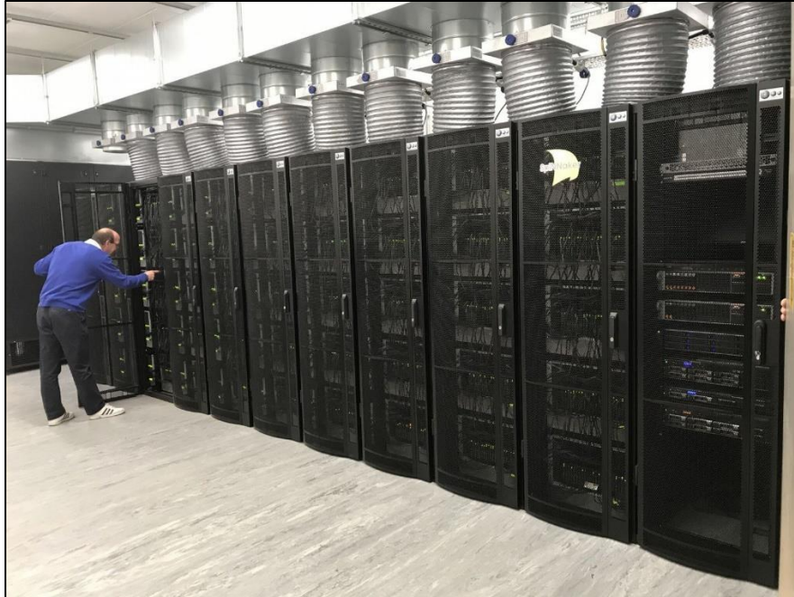
Figure 9 SpiNNaker - Large Scale digital Neuromorphic System (Jordan, 2018)
