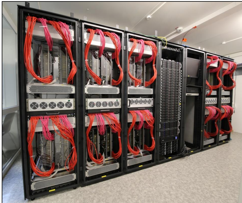
Figure 10 BrainScales – A Large Scale Analog Neuromorphic System
