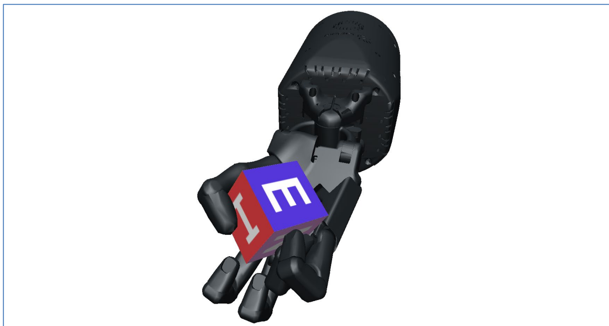
Figure 1: Image of the Shadow Dexterous Hand in the process of manipulating a cube.
