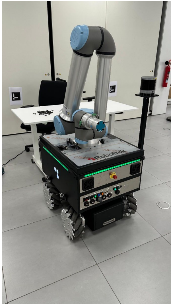
Figure 12: RB-KAIROS robot in ROB performing arm motor action based on working memory
