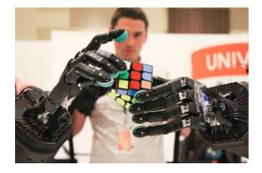
One of the most difficult parts of the human body to imitate due to its complexity is the hand. The Shadow Robot Company designs and develops highly dexterous robotic hands that are as realistic as possible to human hands and makes them available to researchers within the framework of the Human Brain Project. The goal is to integrate them
