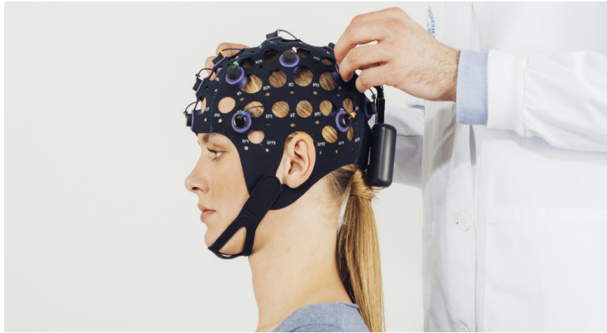
Figure 27. High-quality EEG that records with a resolution of 24 bits at 256Hz for 6+ hours thanks to active shielding with stable sensor contacts. (source: https://www.bitbrain.com/neurotechnology-products/semi-dry-eeeg/versatile-eeeg )
