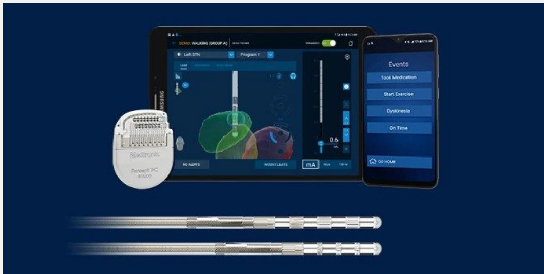
Figure 10. Percept PC Deep Brain Stimulation (DBS) system
