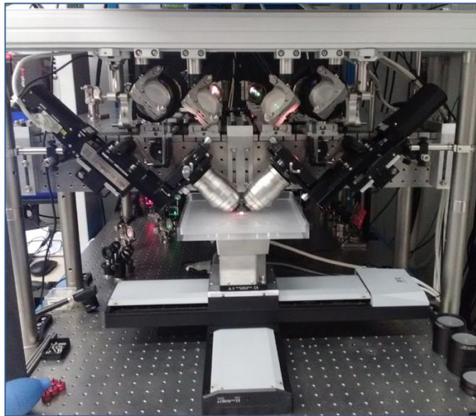
Figure 7: Photo of the inverted ultra-fast large-area light sheet microscope.
