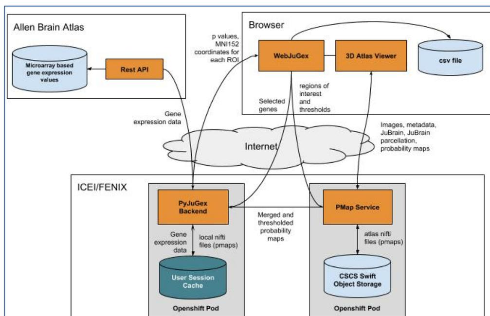
Figure 2: Software architecture of Web-JuGEx integrated in the HBP ecosystem.
