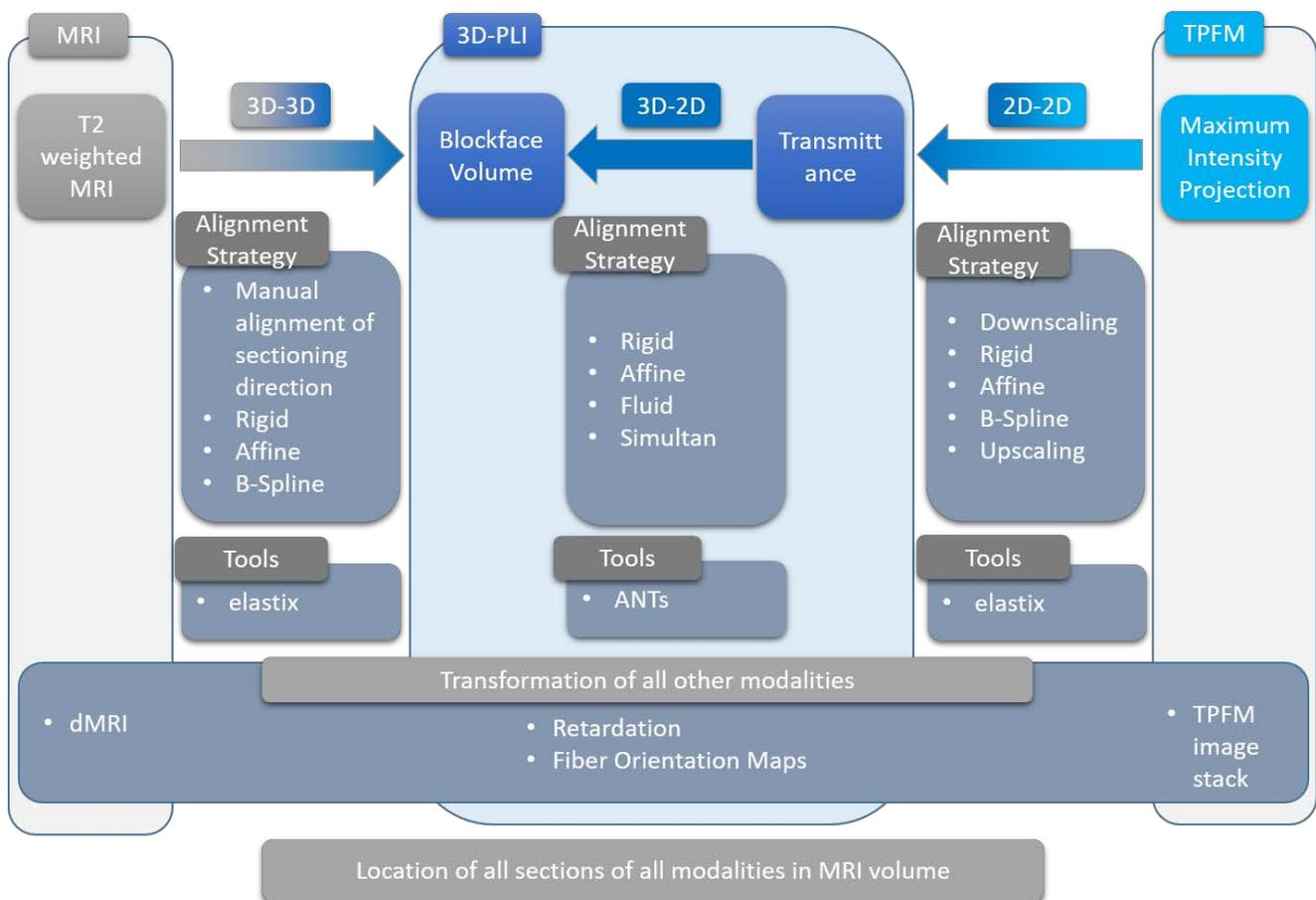
Figure 2: Overview schematic of the developed multimodal co-alignment concept.
