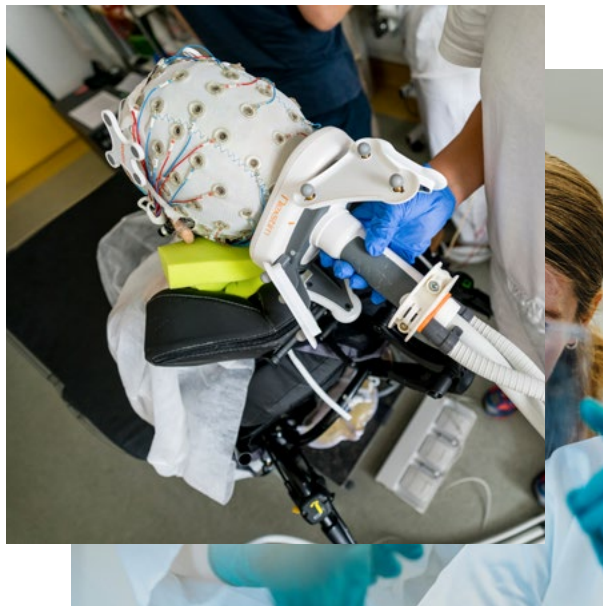
Simultaneous EEG recording and magnetic stimulation
