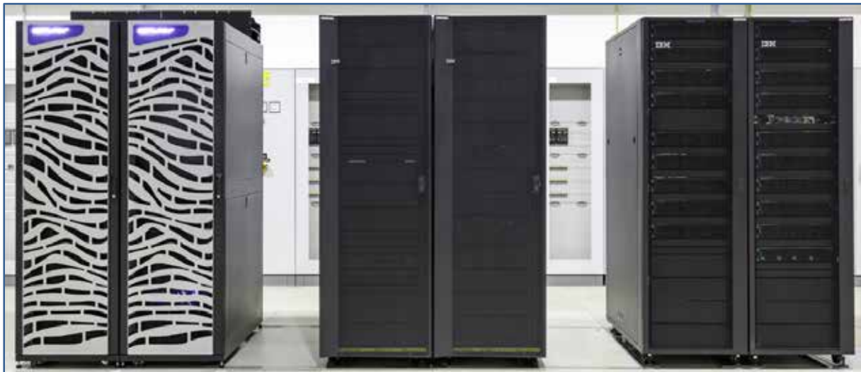
Figure 3: Pilot systems JULIA (left) and JURON (right). The racks in the middle host the shared storage.
