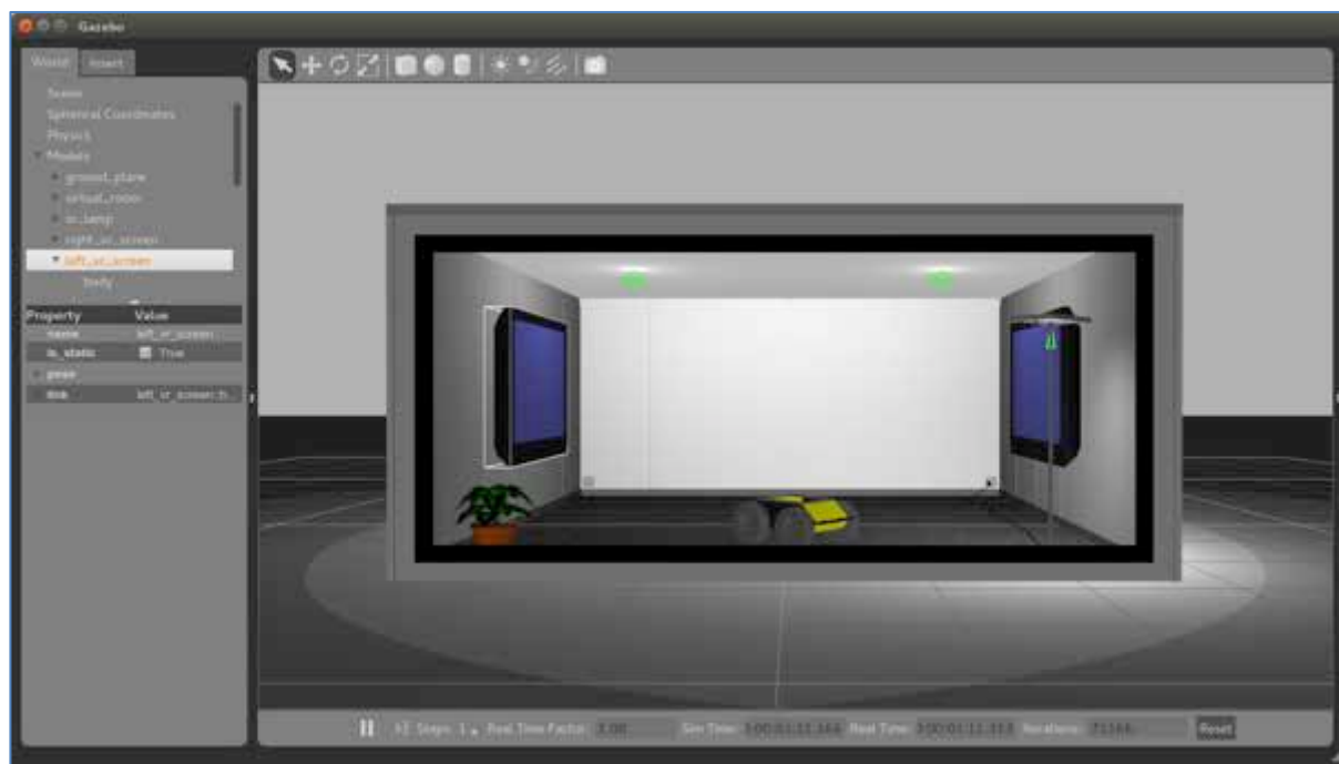
Figure 8: Virtual room model with the Husky robot running in the Gazebo simulator
