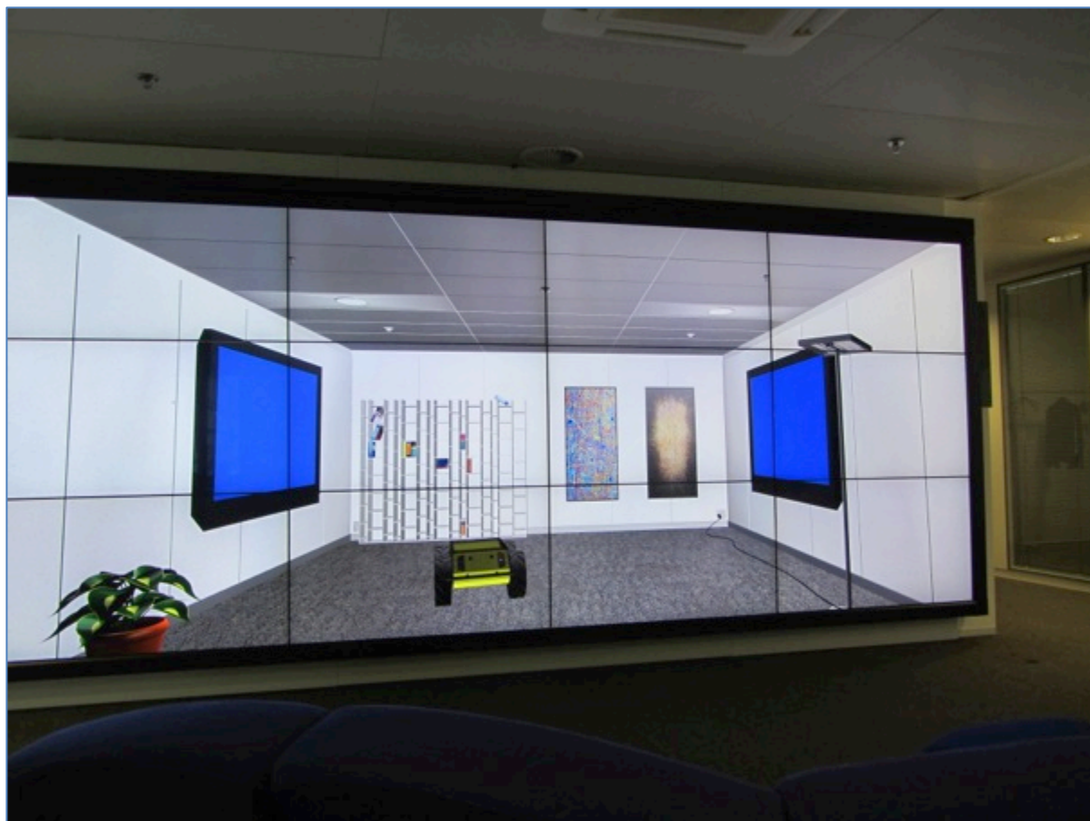
Figure 13: The virtual room experiment running on the EPFL display wall. The display wall is composed of twelve full HD monitors
