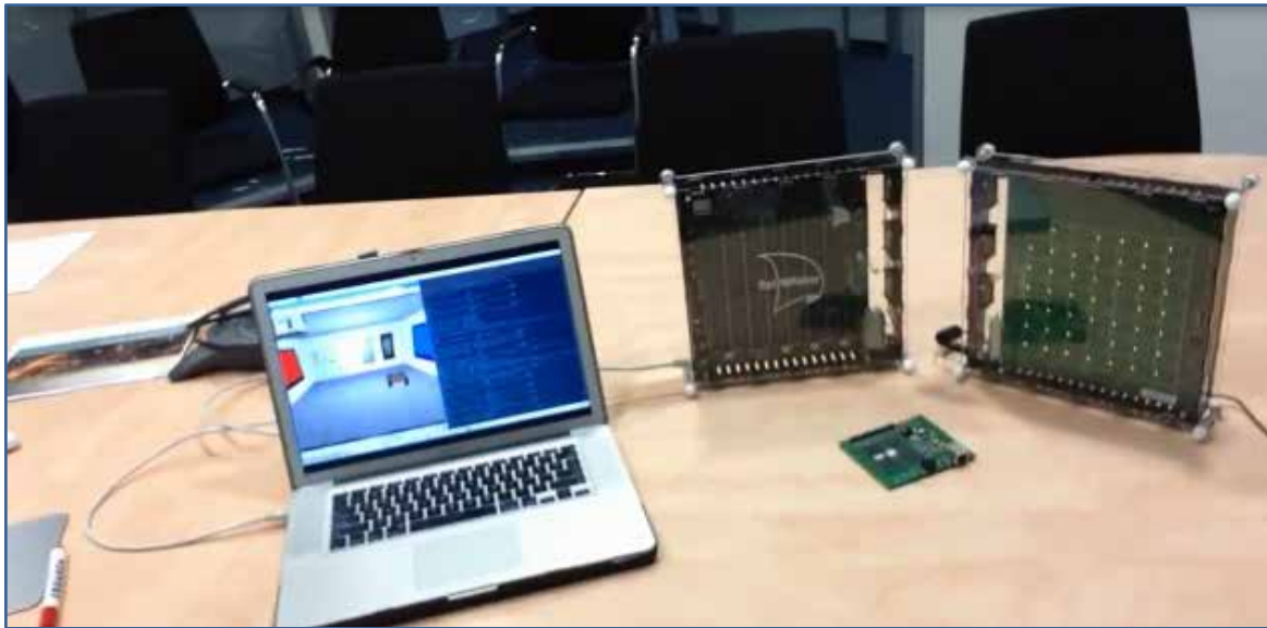
Figure 9: SpiNNaker board running the brain model of Husky-Braitenberg experiment
