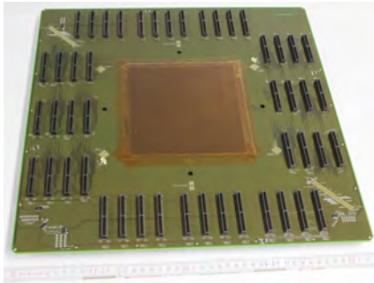
(a) Wafer side with covered pad area and slots for 48 FPGA boards.
