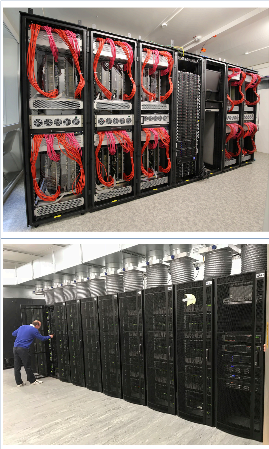
Figure 1: The BrainScaleS (upper image) and SpiNNaker (lower image) machines. These machines form the HBP Neuromorphic Computing Platform, offering accelerated learning and programmable flexibility respectively.
