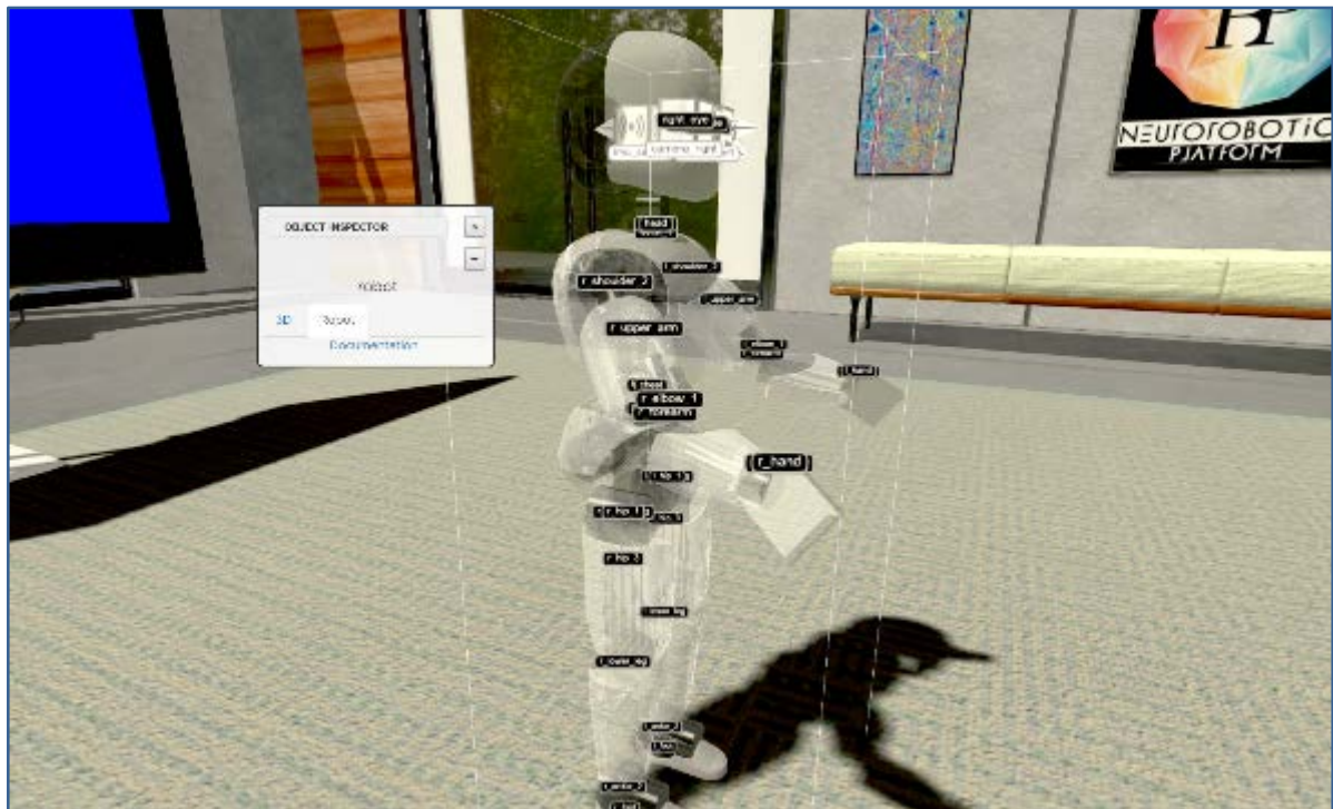
Figure 15: Sensor and actuator labels displayed by the Robot Inspector
