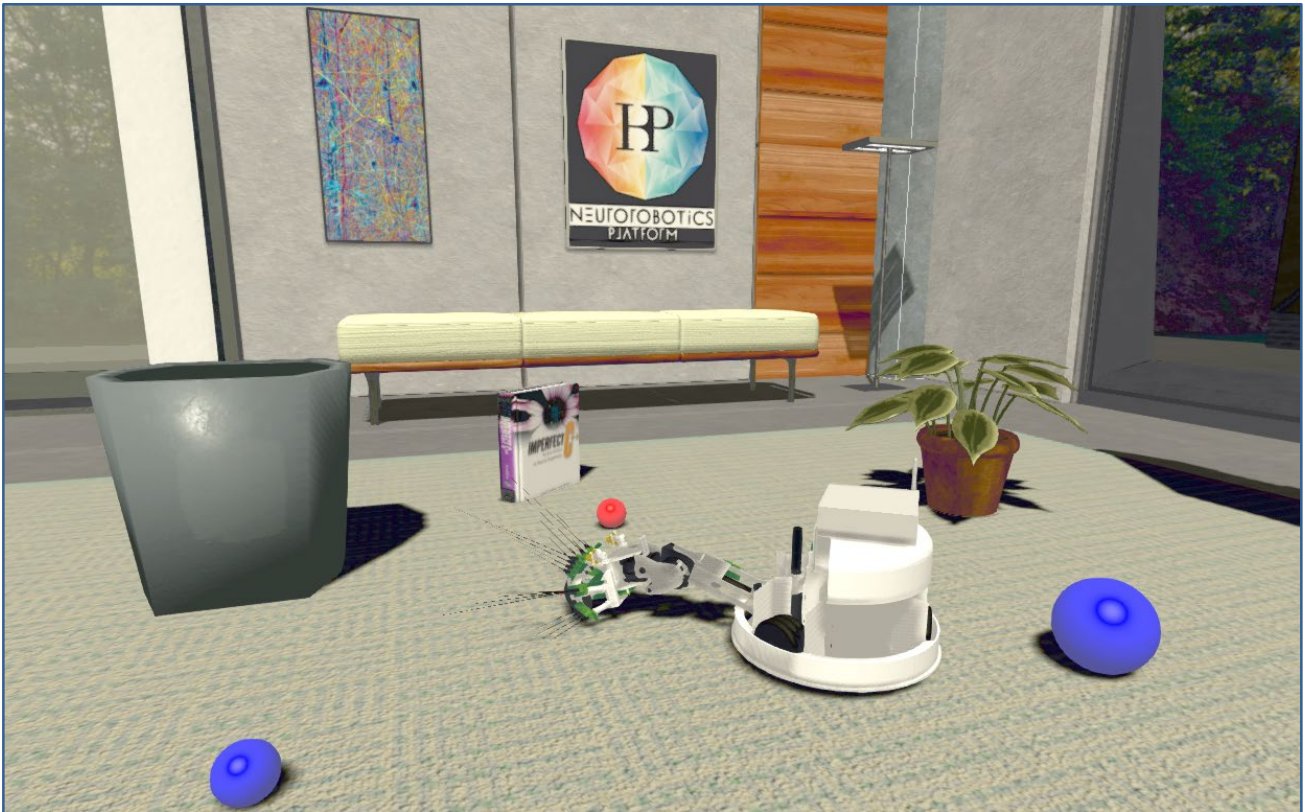
Figure 1: Whiskeye robot explores a virtual environment on the NRP through tactile sensory input
