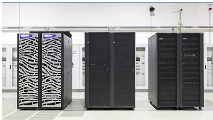
Figure 1: Pilot systems delivered within the HBP's pre-commercial procurement. JULIA (left) has been delivered by Cray and JURON (right) by IBM and NVIDIA. Both systems use a shared high-performance storage system (middle).
